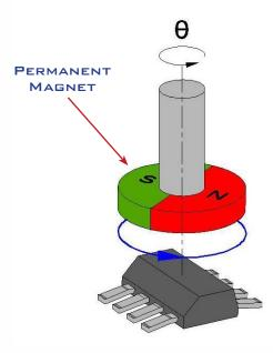
As the MR technology is not needed to have physically all the output lines (poles in case of a magnetic encoder) on the encoder disc, the MR encoder can be made very compact, even for high resolution. The magnetic field inside the encoder can be maximized by having a low number of relatively big magnetic poles. The strong field so obtained makes this encoder very resistant against any unwanted external field.
