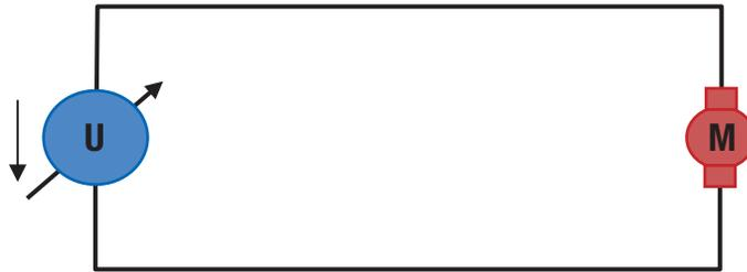
**Figure 1: Driving motor using variable DC source**
